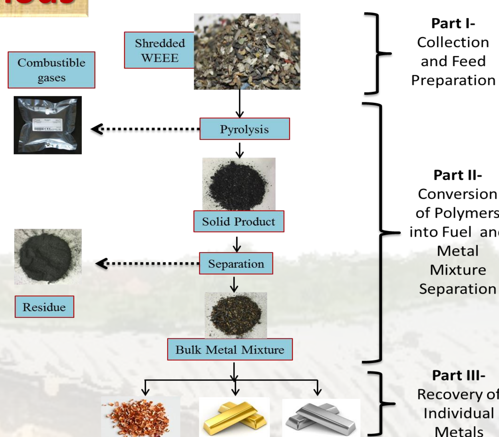
10 kg/h Pyrolysis Pilot Plant (a) Process flow diagram and (b) Composition of gaseous product
